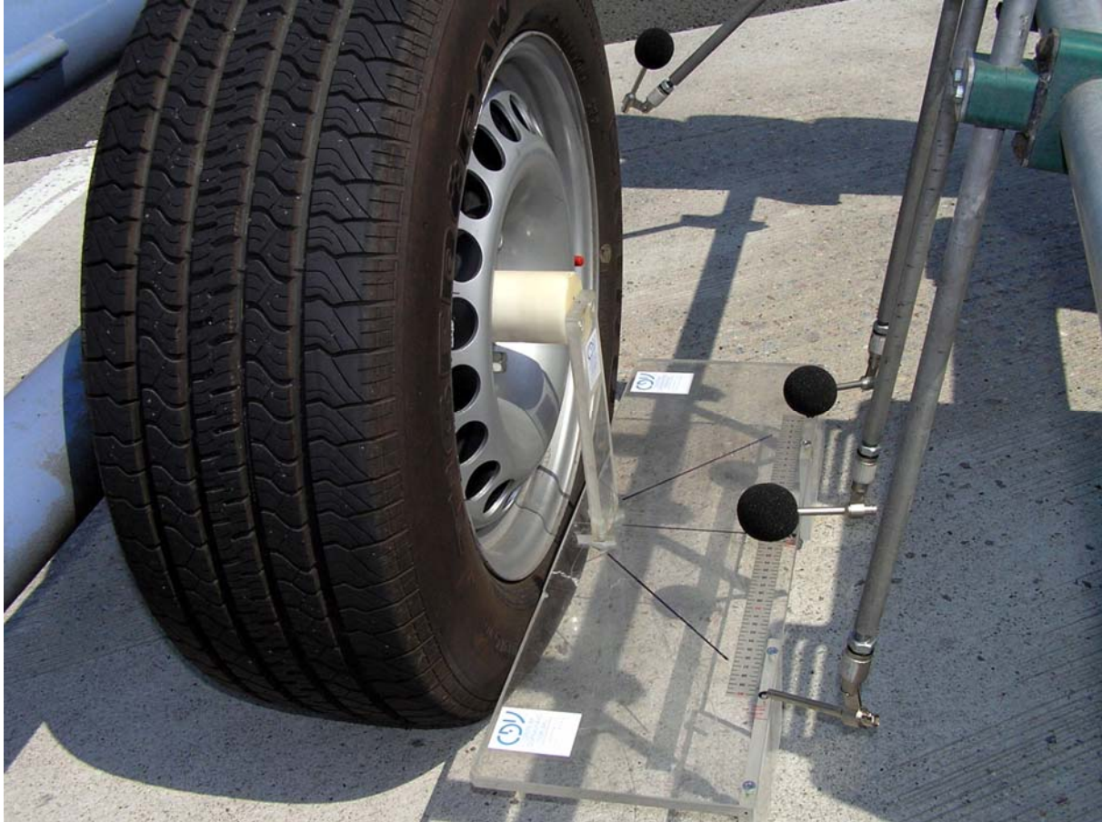
Fig. 4: Setting up the measurement microphones on the testing CPX trailer against the reference tyre SRTT.
