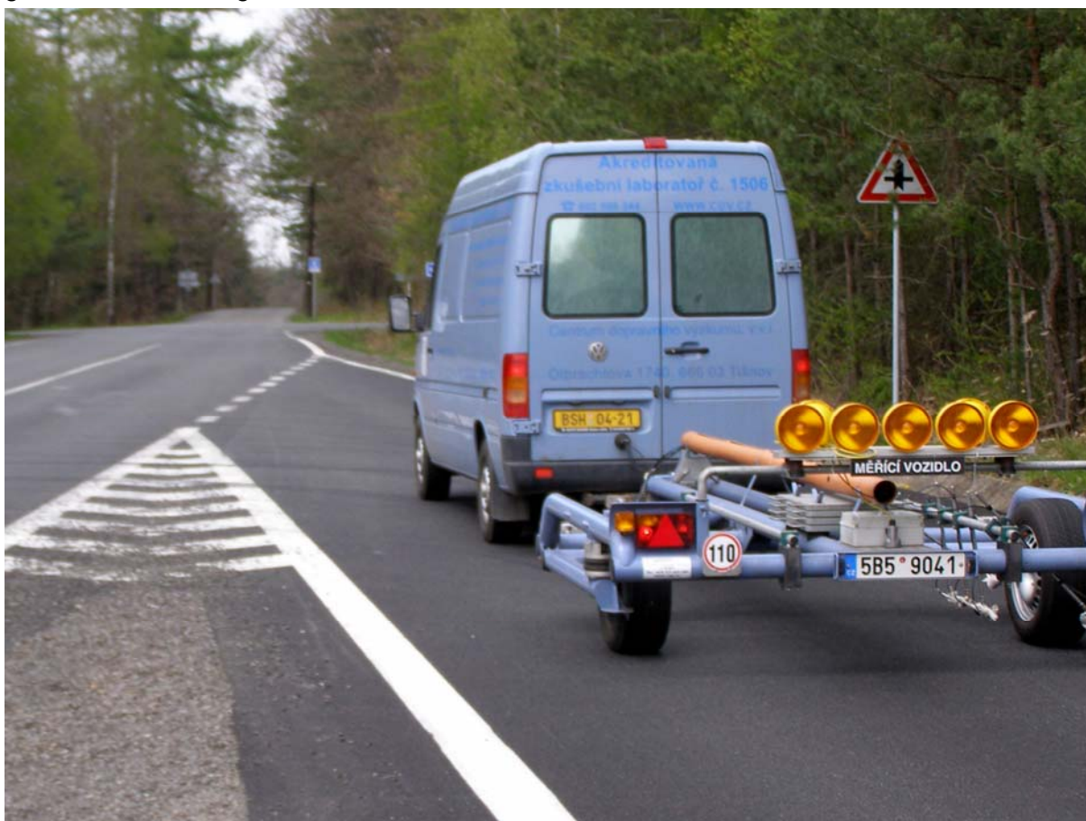
Fig. 5: Look at the measurement vehicle with the testing trailer for the measurement on the given road according to the CPX method.
