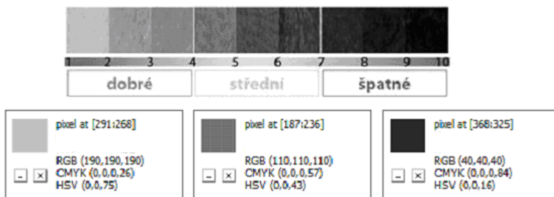
Fig. 1: Limit of wear of motor oil (in grey shades) [9]
