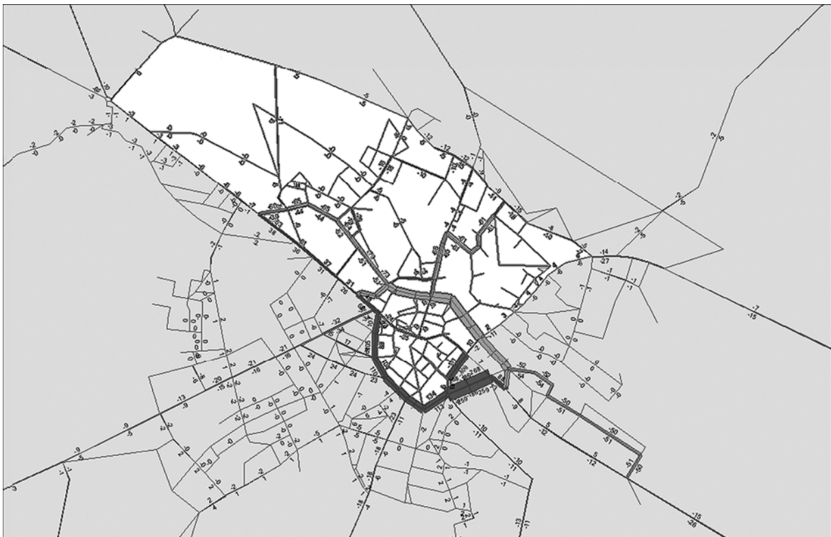
Fig. 3: Difference cartogram of PM emissions - scenario with a greater low emission zone compared to the current state
