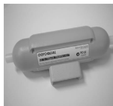
Fig. 3: Removable monitor head
