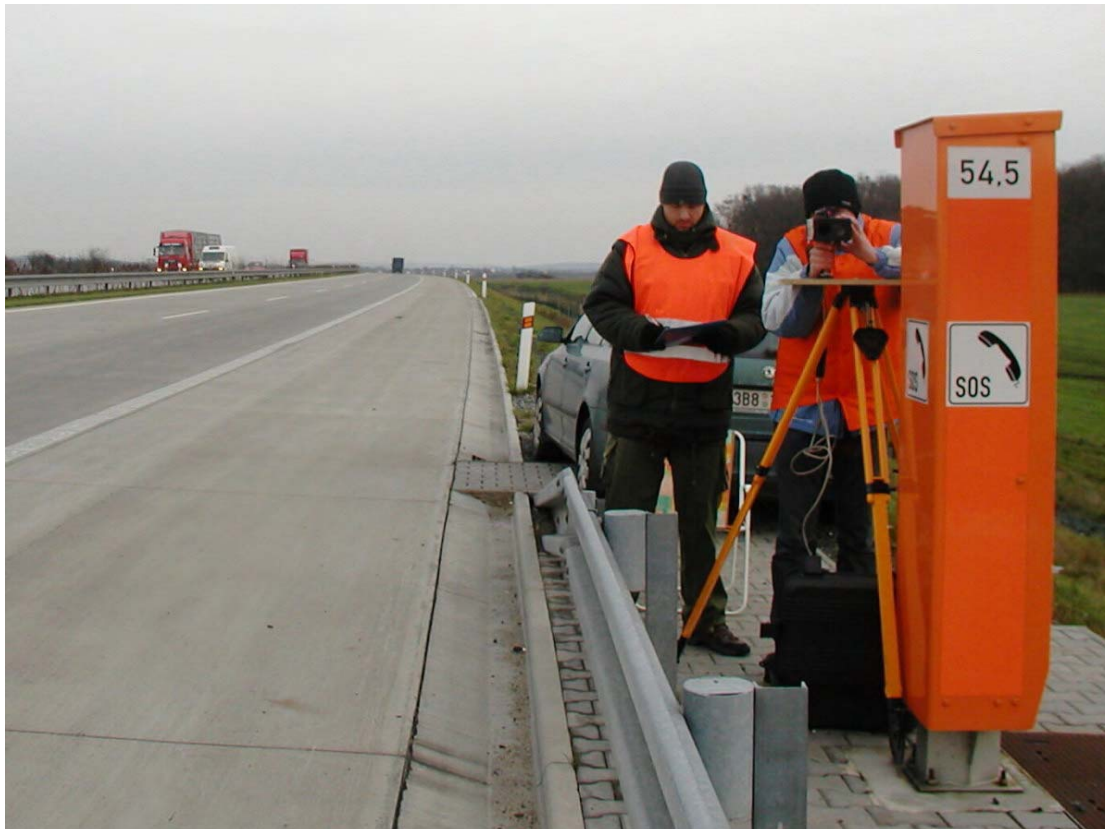
Fig. 1: Measurement of the speed of vehicle pass-bys by the laser gun.
