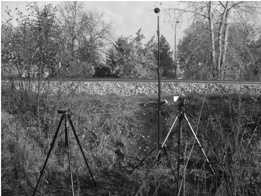
Fig. 5: Sound pressure measuring equipment
