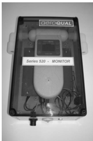
Fig. 1: Aeroqual 520 Monitor, adjusted for the external use
