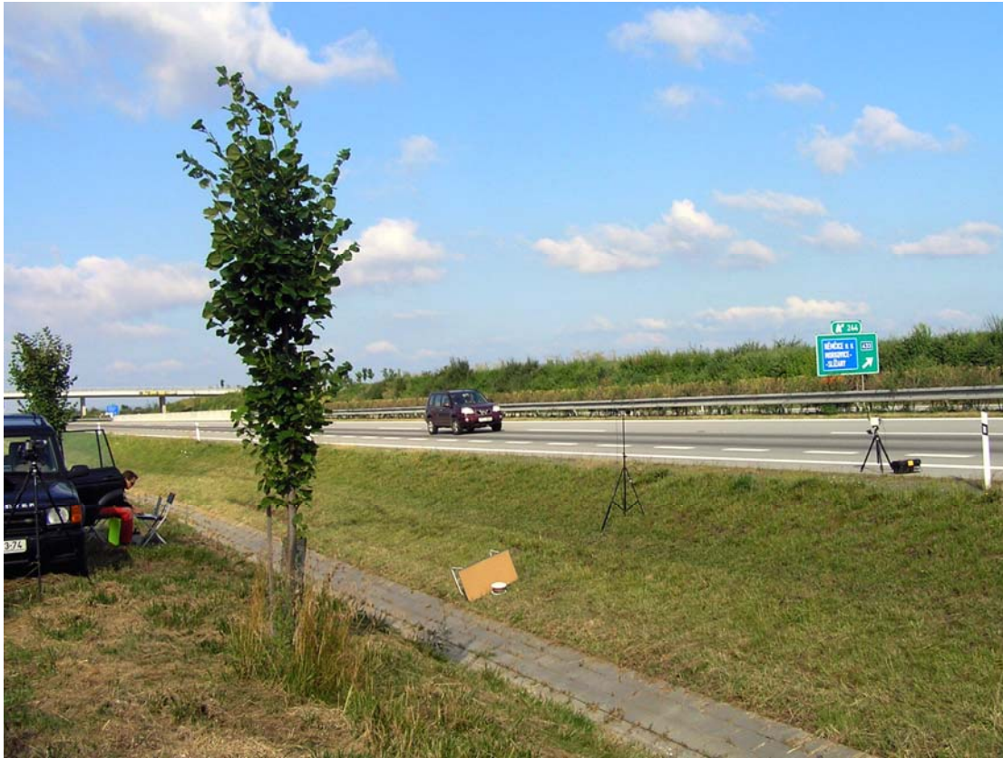
Fig. 2: Measurement chain for the SPB method applying the radar with the wireless data transfer.
